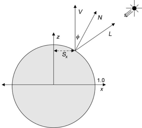
**Figure 3: Estimating lighting direction from a highlight location on the surface of a glossy sphere assuming a distant camera.  $V$  is the view vector pointing to the camera,  $N$  is the surface normal,  $L$  is the unknown, normalized light vector we solve for.**
