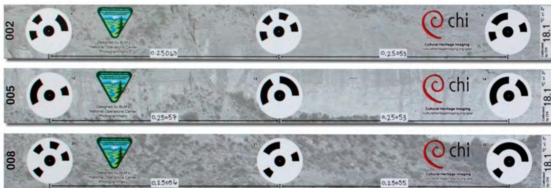
Include 3 coded targets. Centers of each target are approximately 25cm apart, with a total distance from targets at each end of 1/2 meter (or 50cm). The bar's overall dimensions are 60cm long x 6cm wide.
