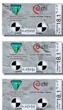
Include 2 non-coded cross-type targets. Centers of each target are approximately 5cm apart. The bar's overall dimensions are 10cm long x 6cm wide. Scale bars with non-coded targets can be useful when imaging small subjects.
