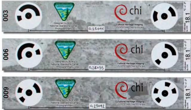
Include 2 coded targets. Centers of each target are approximately 25cm apart. The bar's overall dimensions are 35cm long x 6cm wide.
