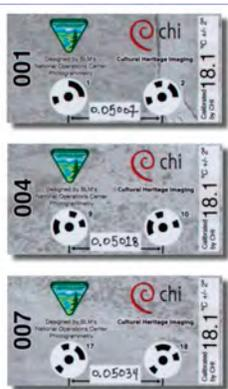
Include 2 smaller coded targets. Centers of each target are approximately 5cm apart. The bar's overall dimensions are 10cm long x 6cm wide. The smaller target diameters can be helpful when documenting smaller subjects.
