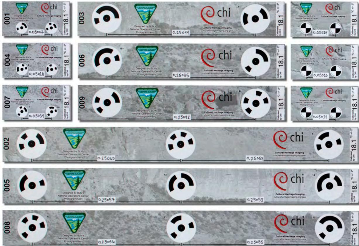
The 12 scale bars in the set are flat, lightweight, linear bars. These are calibrated scale bars with printed targets separated by a known distance. There are three each of four sizes/styles, 9 coded, 3 non-coded.
